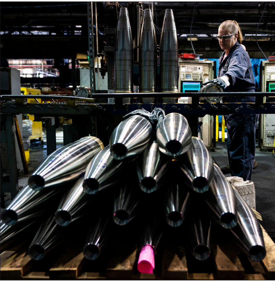
A steelworker moves a 155 mm M795 artillery projectile during the manufacturing process at the Scranton Army Ammunition Plant on April 13, 2023. ASSOCIATED PRESS FILE
