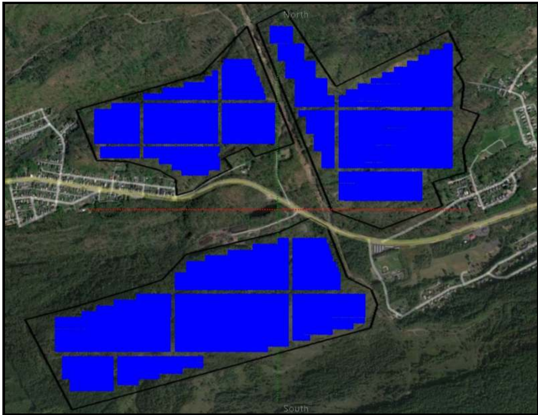
Tracker Modeling - Full Array - ~114 MW-AC
