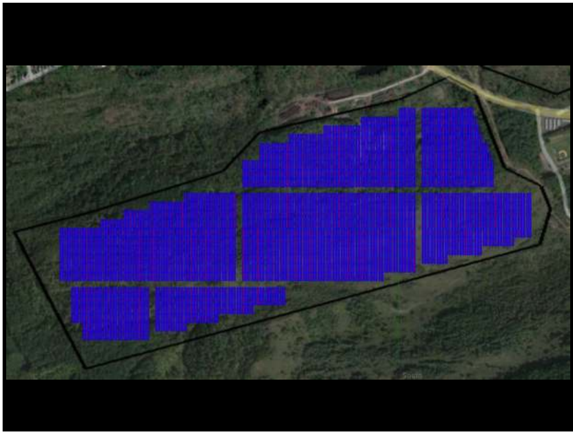
Tracker Modeling - South West Array - ~52.5 MW-AC
